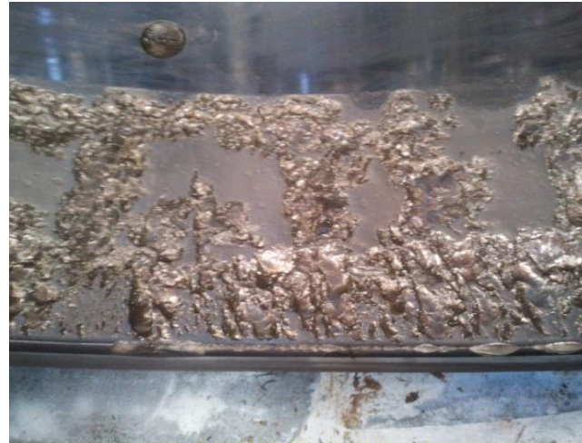
A damaged main bearing of a wind turbine – Courtesy of Engie Green / Damien Bruyère
