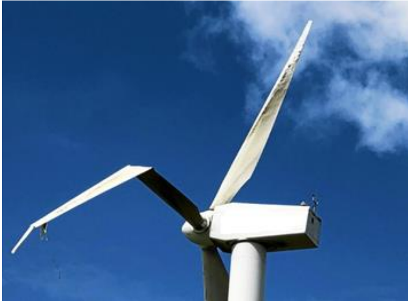
A wind turbine with broken blades – https://bit.ly/33JOyAf
