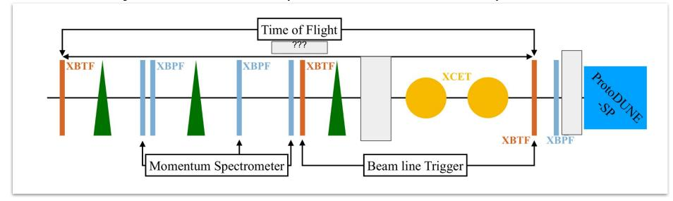
Only 1 profile monitors in the downstream section → No track reconstruction/projection to the beam Rest of layout is relatively the same (modulo lengths)
