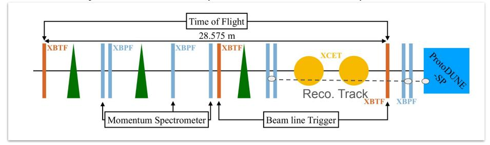
Blue lines: 192-channel scint. fiber monitors. 1D Profiles (2 orthogonal →2D Profile)
