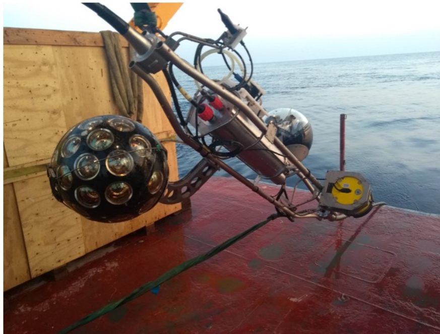
The recovery of the PPM-DOM, the first prototype of the future KM3NeT DOMs, still in good shape. This marks the passage to the next generation - KM3NeT.
