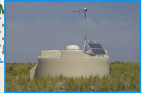
1665 surface detectors: water-Cherenkov tanks (grid of 1.5 km, 3000 km<sup>2</sup>)
