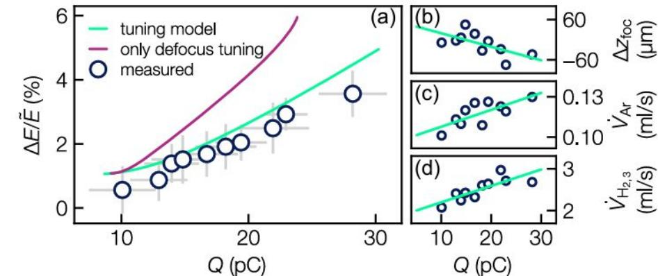
Beam charge tuning curve at 250 MeV
