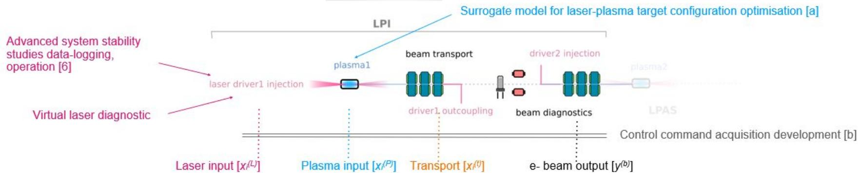
In the context of advanced accelerator high quality beam laser plasma injector (LPI) for EuPRAXIA [1] preparatory technical design phase and future high gradient accelerator R&D at IJClab [2]: 10 Hz **200MeV** LPI test facility to improve quality and stability of e- beam generated by laser-plasma accelerator.
