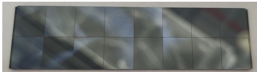
Bump Bonding Process Verification with Dummy Dies
