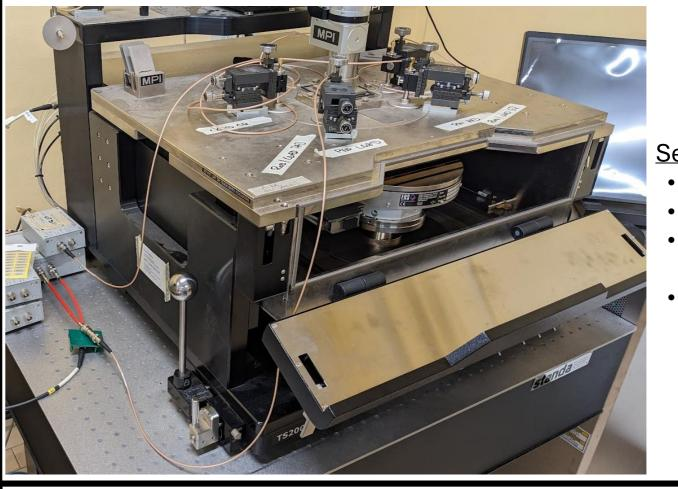
Setup: Environmental isolated enclosure Thermal chuck [-60°C , +250°C] Metallic needles attached to micromanipulators • Device analyser for automatic and precise measurements
