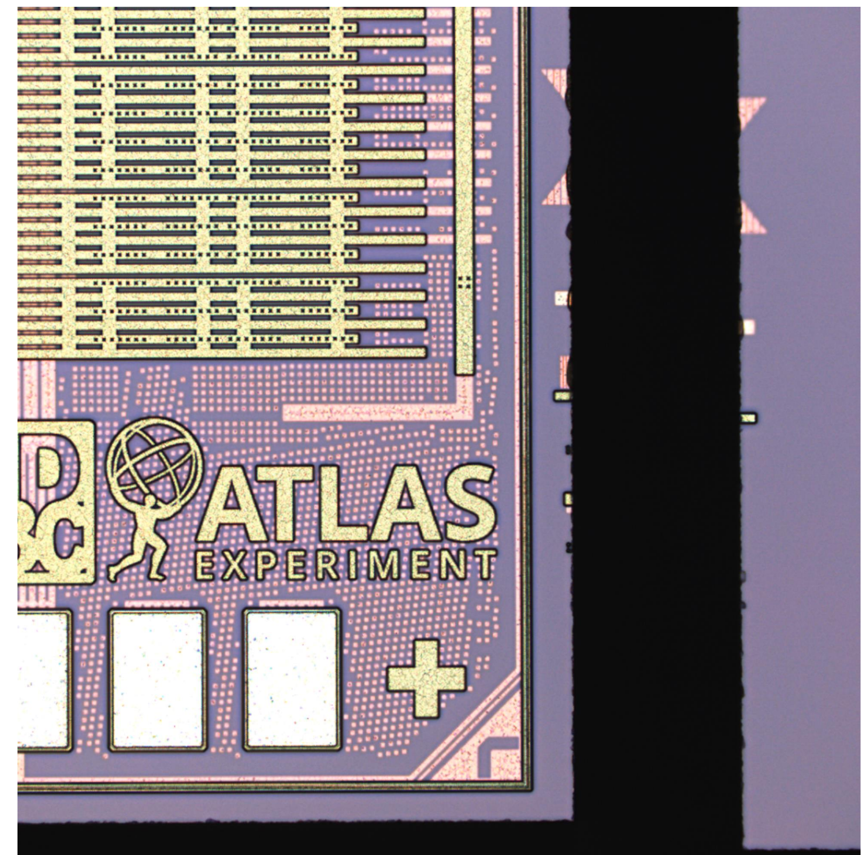
Diced wafer chip edge with wire bond pads (bottom left) and digital chip bottom (top left) (credit to Maurice Garcia-Sciveres)
