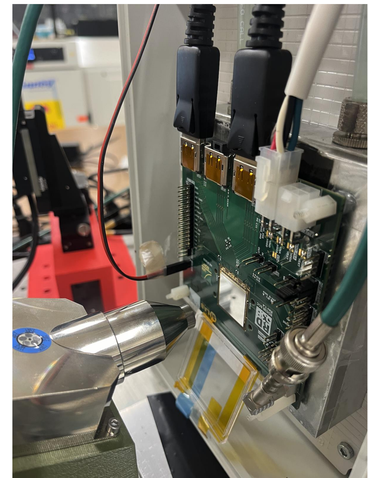
X-ray tube aligned with chip high-rate studies
