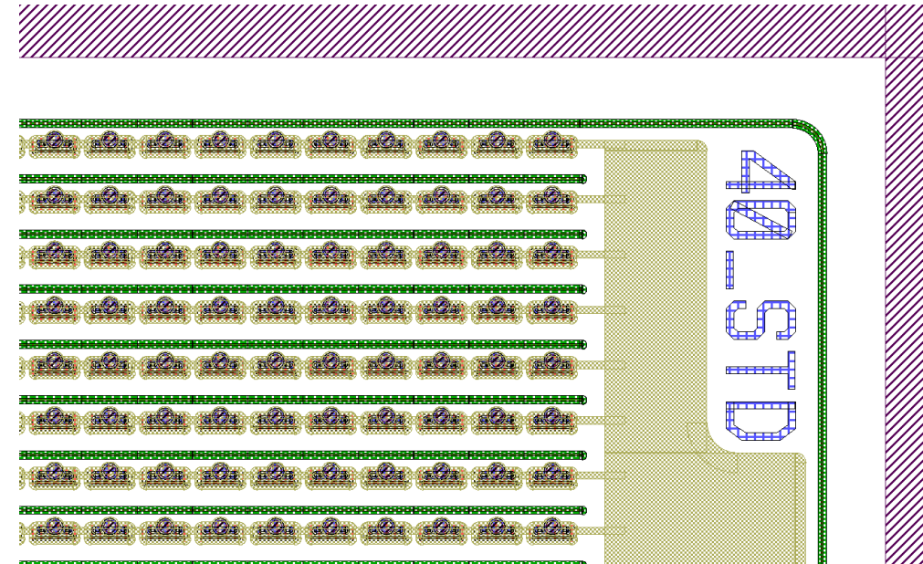
Layout of 64×64 sensor (STD design) Only the corner region is shown
