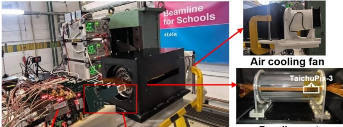
Baseline vertex detector prototype
