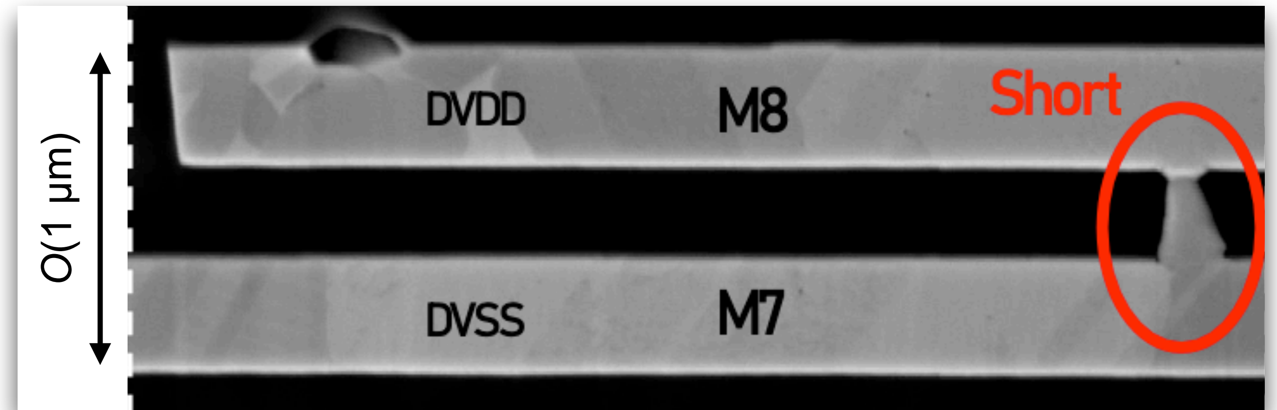
SEM cross section of the top two metal layers
