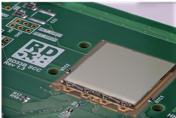
ITkPixV1 on a single chip card
