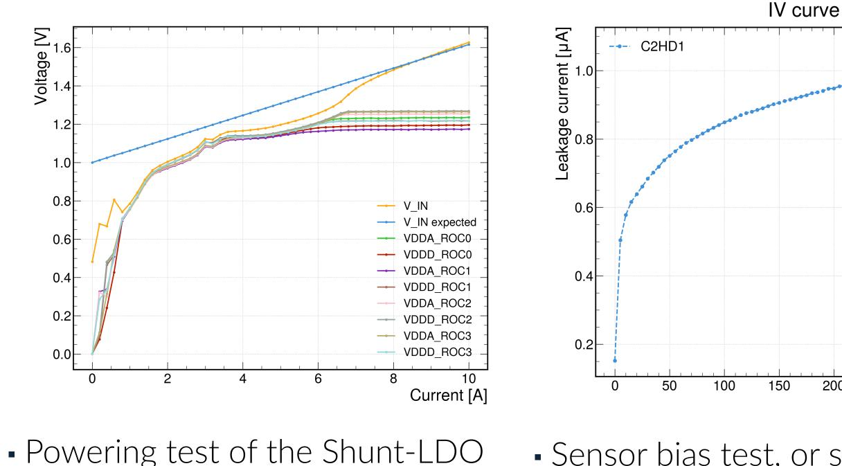
circuit of the readout chip (ROC)
