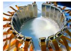
Title: Silicon Drift Detectors of the SIDDHARTA-2 experiment for X-ray spectroscopy of kaonic atoms
