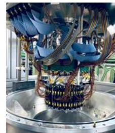
Title: Internal view of the SIDDHARTA-2 experimental setup, showcasing the intricate arrangement of detectors and cabling.
