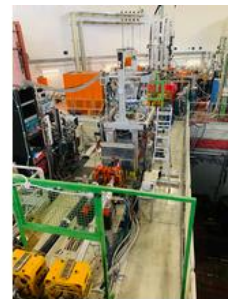
Title: Photo of the SIDDHARTA-2 experimental setup at the DAFNE collider, showing the apparatus installed above the electron-positron interaction point.
