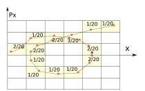
Trajectory starting from a given cell of the phase space, calculated for 20 time steps.
