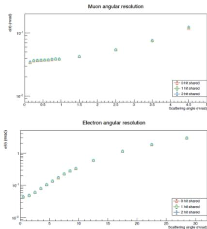
Angular resolution as a function of the scattering angle for the outgoing muon (top) and electron (bottom), obtained by fitting the residual distribution of the reconstructed angle using MC truth.
