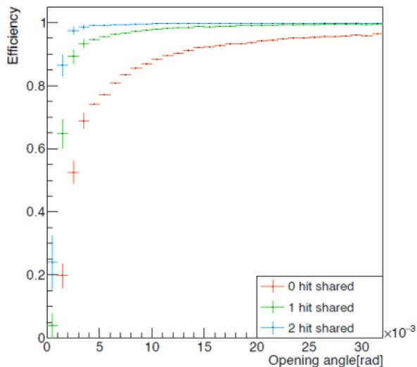
Reconstruction efficiency for the elastic event as a function of the  $e - \mu$  opening angle.
