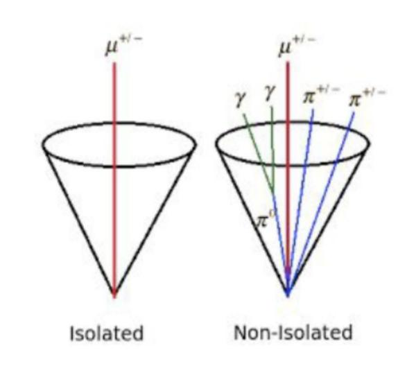
For the second level of software trigger the group has developed general tools needed for filtering the events and also usable at the level of the offline analysis. This includes, for examples, developing the algorithm for evaluating the particles isolation, a powerful tool for background suppression. Selections for physics analysis have been designed and implemented, putting the basis for the exploitation of the Run3 dataset.
