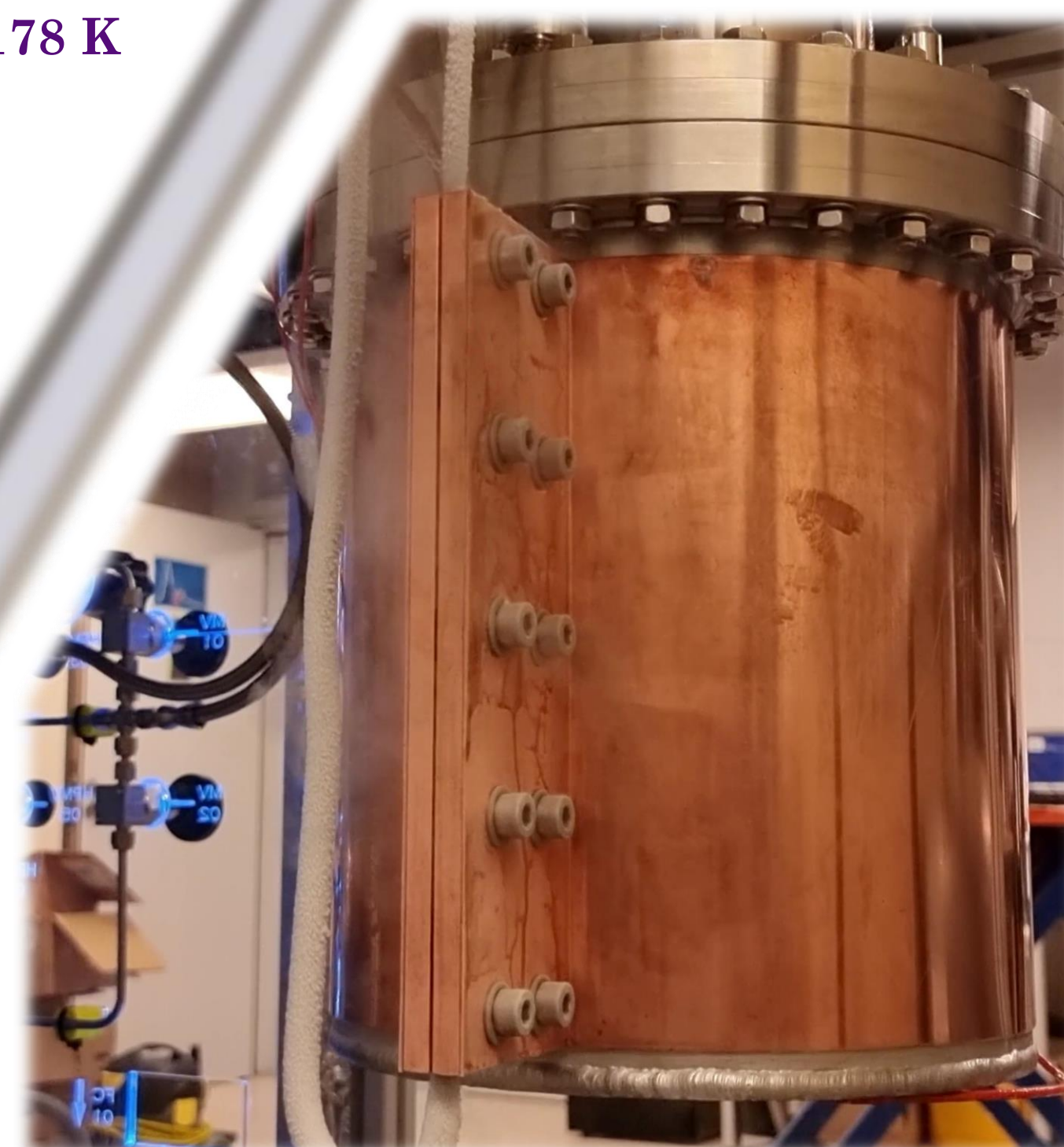
Inner vessel cooling test with LN 2
