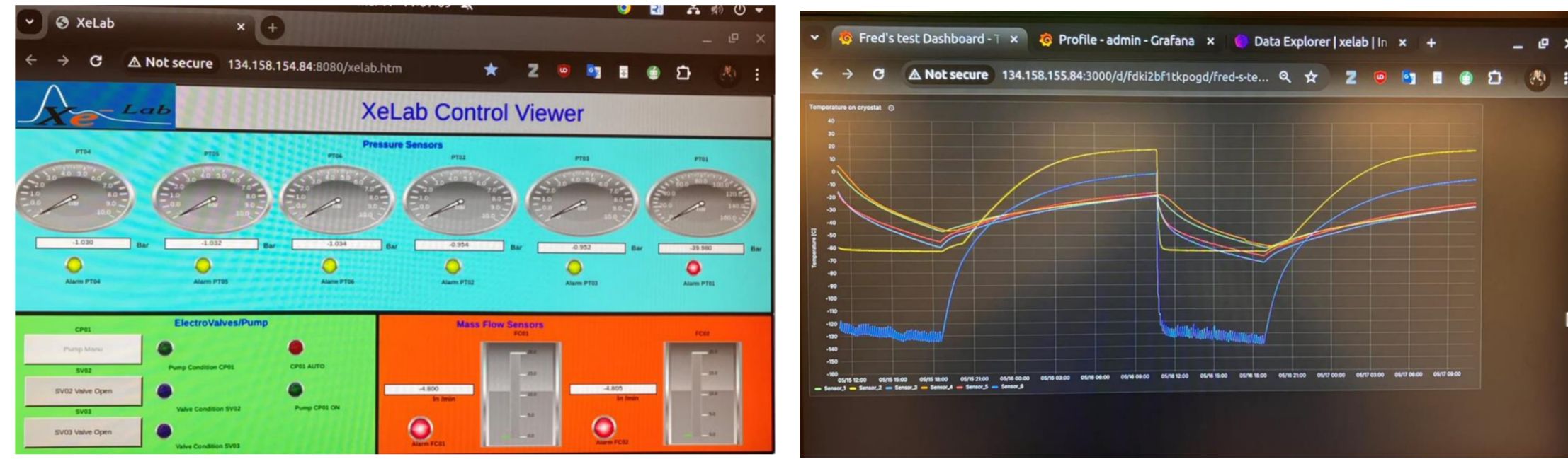
Gas system status with RevPi controlled instrument
