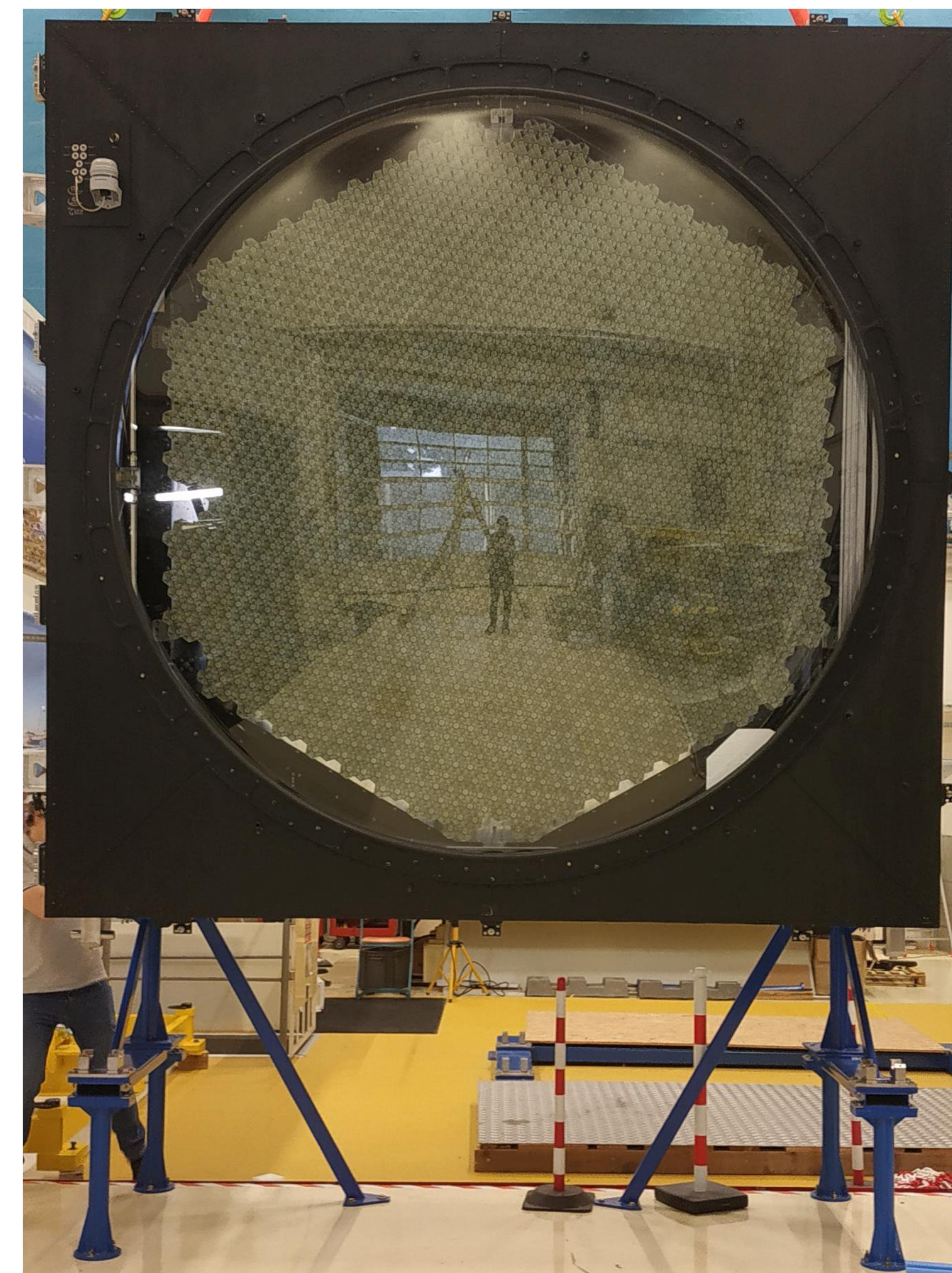
NectarCAM Qualification Model completely equipped with last version of FEB @ Irfu
