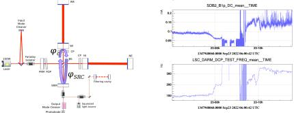
Resonant sideband extraction - TEM00 anti-resonant in signal recycling cavity
