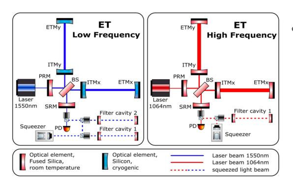
Current proposal: to use two filter cavities for the ET-LF (with detuned SR)
