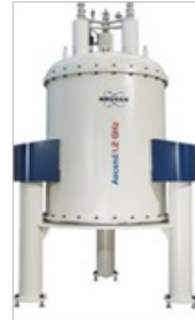
Bruker ASCEND 1.2 GHz 28.2T (LTS/HTS @ 1,9K) 54 mm bore Strongest commercial NMR
