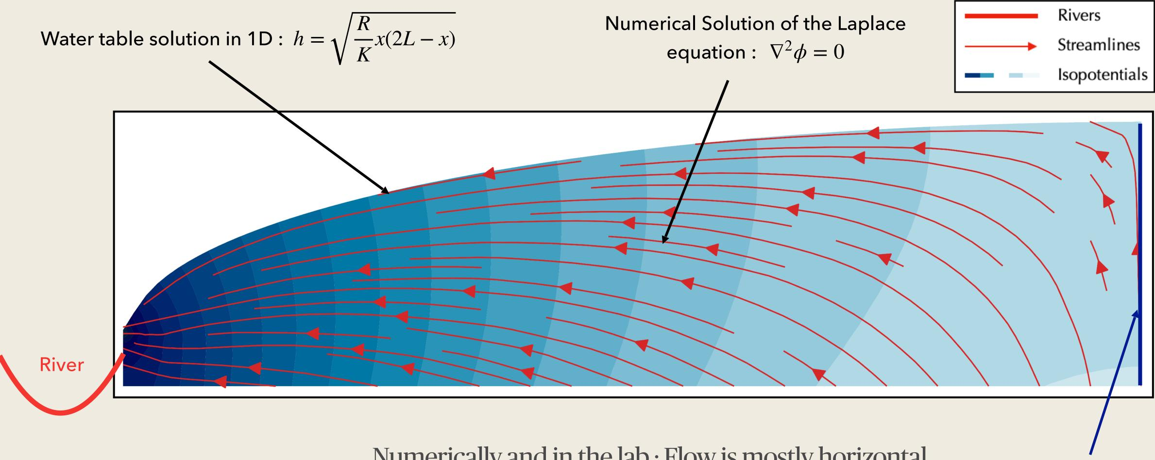
Numerically and in the lab : Flow is mostly horizontal - let's solve over a whole network in 2D
