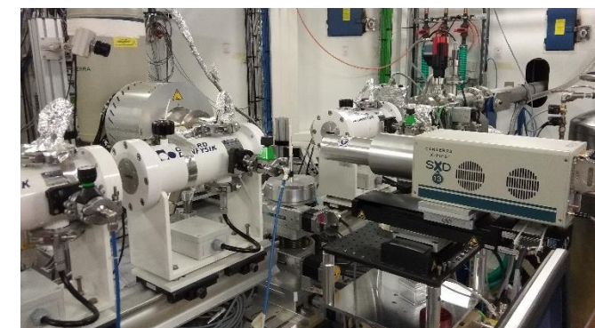
CANBERRA 13EM SDD detector with Xpress3X DPP at SAMBA beamline
