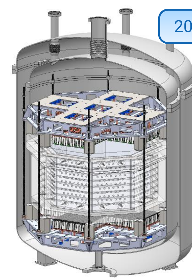
Darkside-20k experiment under construction at LNGS using FBK SiPMs fabricated at Lfoundry: 20 m 2 of SiPMs operated at 87 K.
