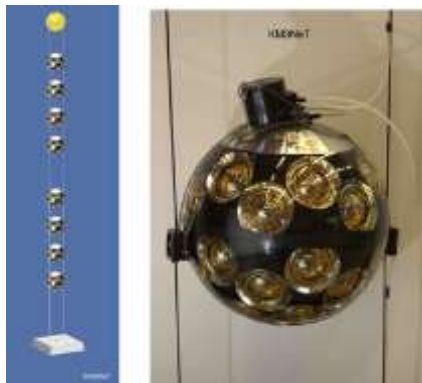
Figure xx : Detection string schematic and DOM
