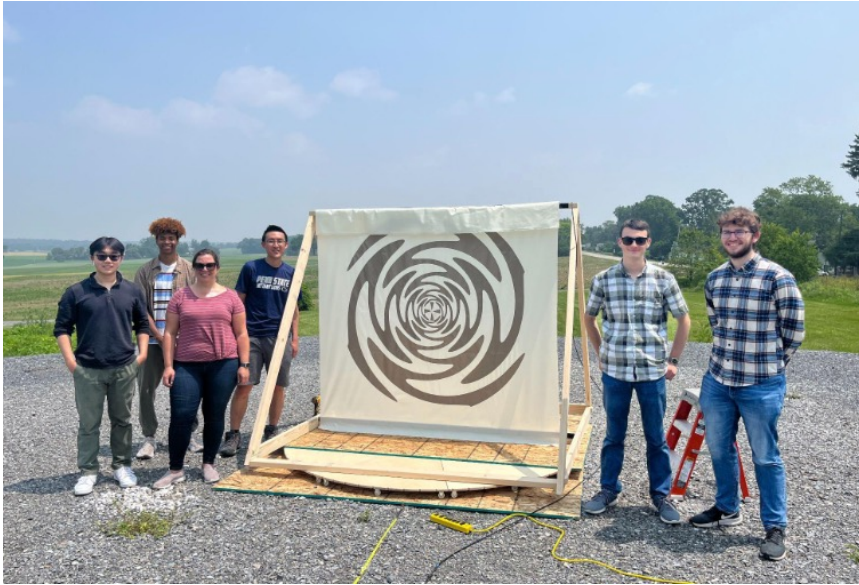
Dual-polarized sinuous antennas, 50-300 MHz.
