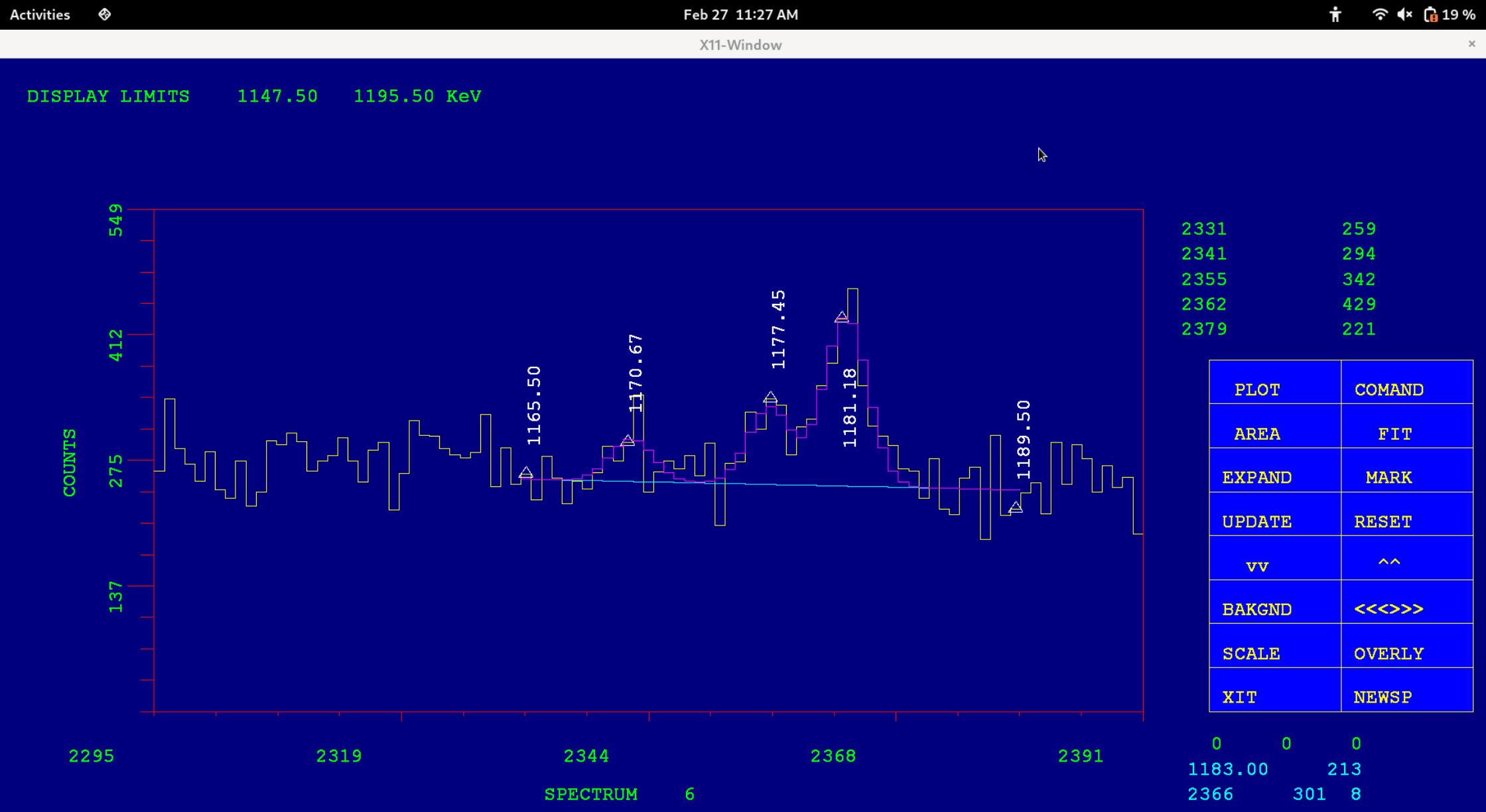
Tripe gamma coincidence: Gate on 431-982 keV + Gate on 274 -410 keV
