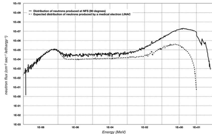
Simulated energy distribution of neutrons available for sample irradiation at SPIRAL2/NFS, compared to the estimated distribution of neutrons produced by a radiotherapy electron accelerator.
