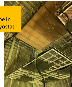
UV photon detectors on cathode and cryostat walls
