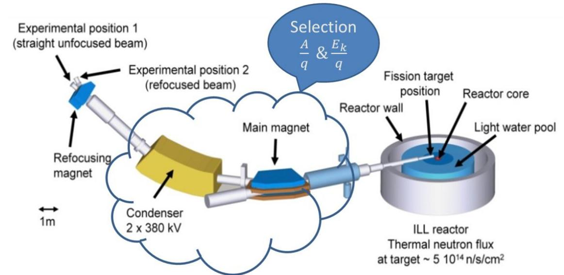
**Lohengrin** : selection with the mass over ionic charge  $\frac{A}{q}$  and Kinetic energy over Ionic charge  $\frac{E_k}{q}$  ratios
