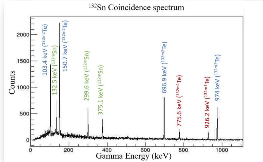
Coincidence between ionization chamber and  $\gamma$  detectors
