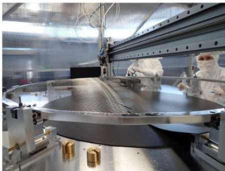
Sid (LPNHE) during the procedure of passivation of electrodes
