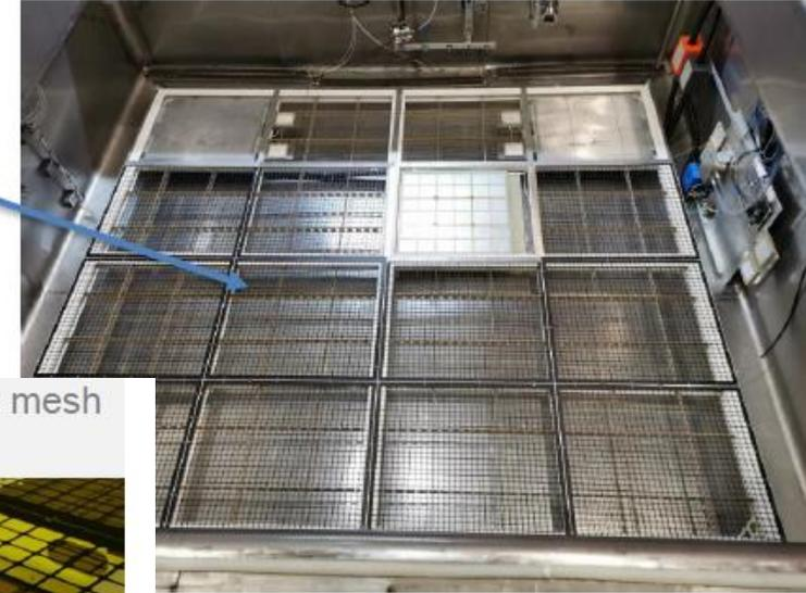
Latest version of resistive mesh on Module-0 cathode
