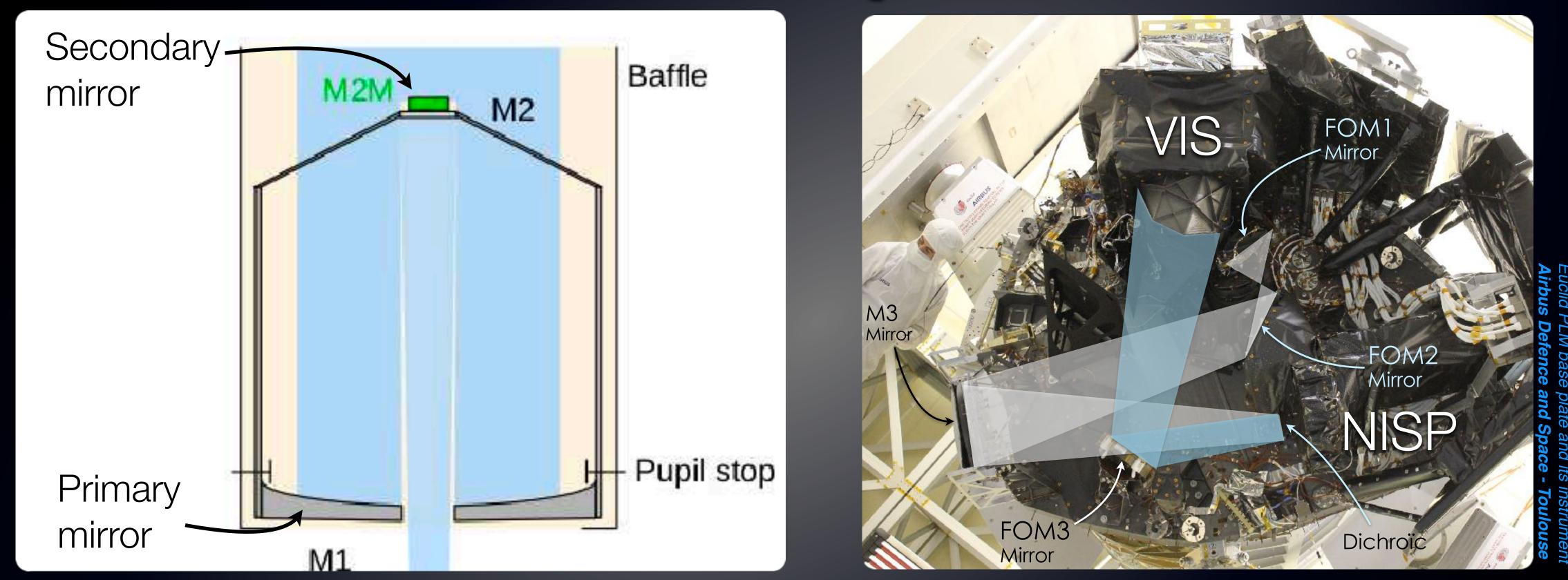
The folding 3-mirrors design corrects for spherical aberration, coma, astigmatism, and field curvature. **Baffle** ensures minimize out of filed stray-light.
