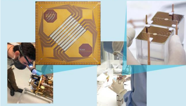
Figure 1. (left) A microscope image of a 128-pixel aluminum-based superconducting tunnel junction array prototype for Phase-IV of the BeEST experiment. This type of array is implanted with large doses of radioactive beryllium-7 and operated at near absolute-zero temperatures to search for exotic new physics [549-50]. (right) A CUPID scientist assembling cryogenic sensors based on scintillating crystals for quantum-enabled light detection [531-52].
