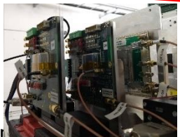
Figure 8.13: Seven 17" silicon ASIC modules, equipped with SKIROC CMS ASIC, mounted on a copper support (cooling phase during the 2017 LHC restart campaign). FCC-France 24
