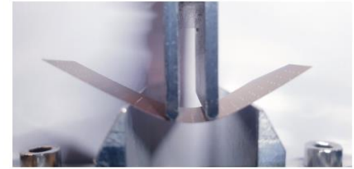
Figure 4.42: Setup for the bending strength measurements.
