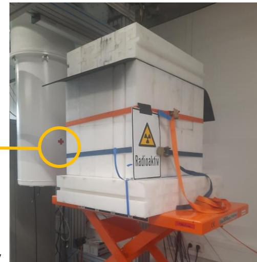
Portable "thermal" neutron source:
