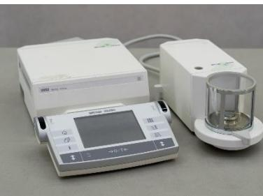
Weighting of pycnometer for traceability of the deposited mass (~ 10 mg)
