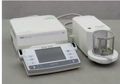
Weighting of pycnometer for traceability of the deposited mass (~ 10 mg)
