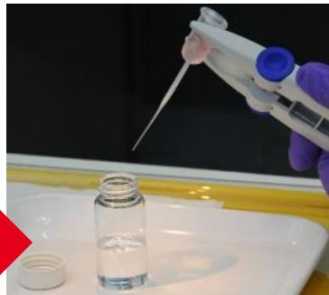
Deposition of solution using a pycnometer
