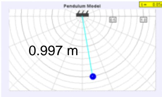
Gravity is not constant on Earth. To get 2 s the pendulum length is actually 99.7 cm
