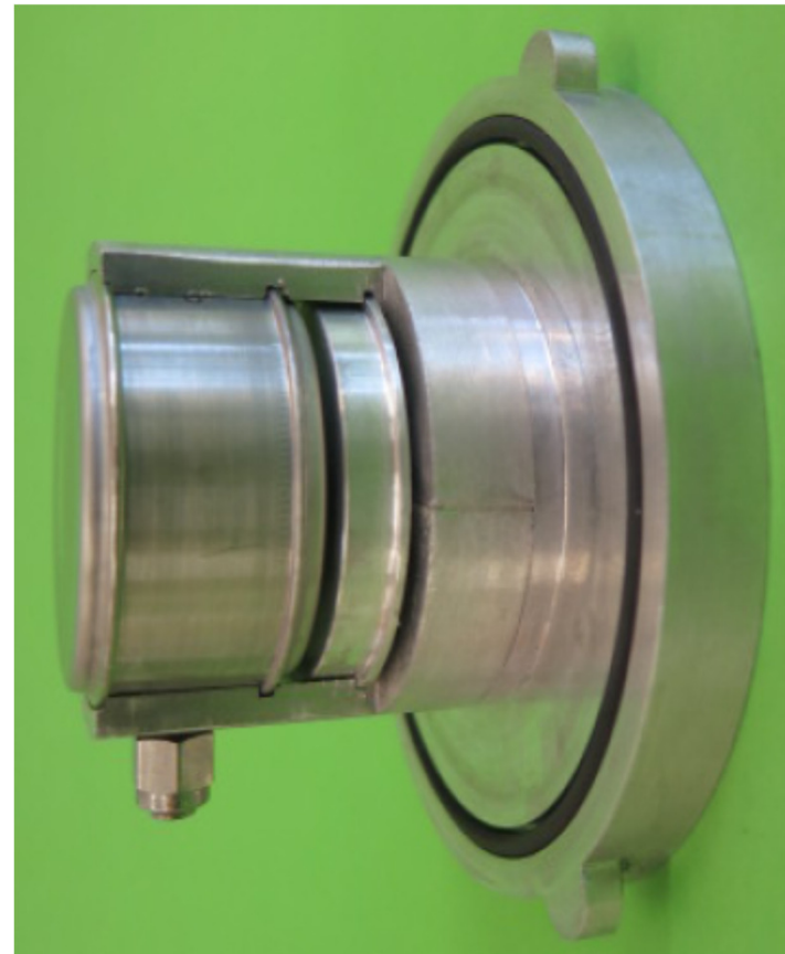
Figure 6. The tandem Rb/Ga targets mounted on a bayonet-mount plug. Instruments 2018, 2, 29; doi:10.3390/instruments2040029
