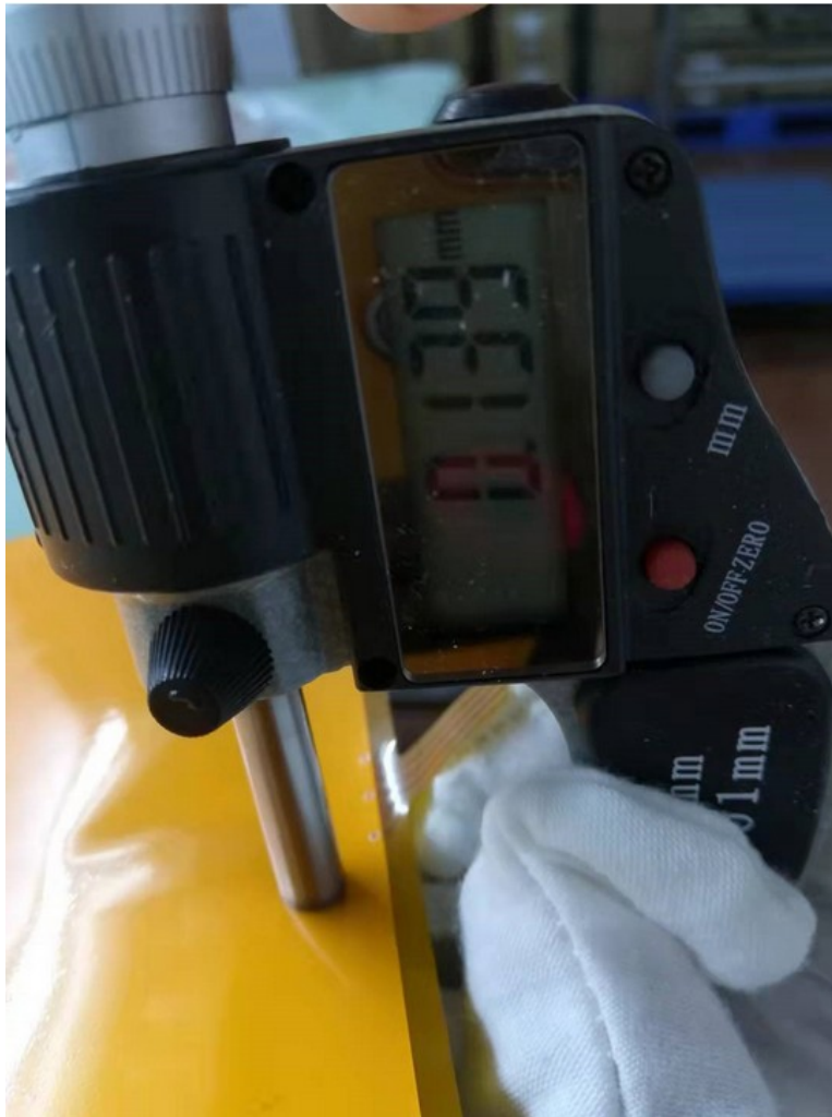
- Flexible thickness without stiffener: 0.139 mm - thickness with stiffener is 0.271 mm
