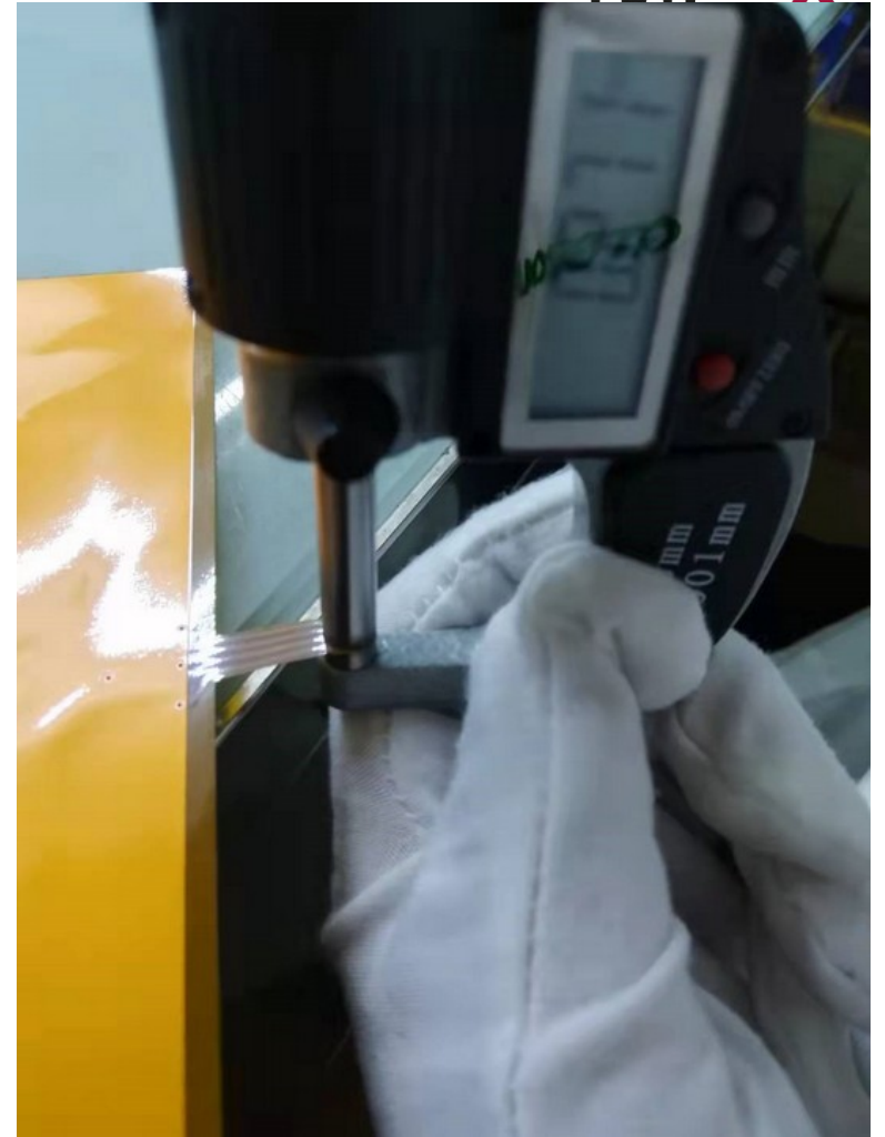
- Flexible thickness without stiffener: 0.139 mm - thickness with stiffener is 0.271 mm
