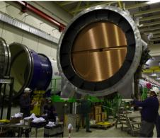
• Liquid Krypton calorimeter (LKr): electromagnetic calorimeter filled with about 9000 l of liquid Krypton at 120K
