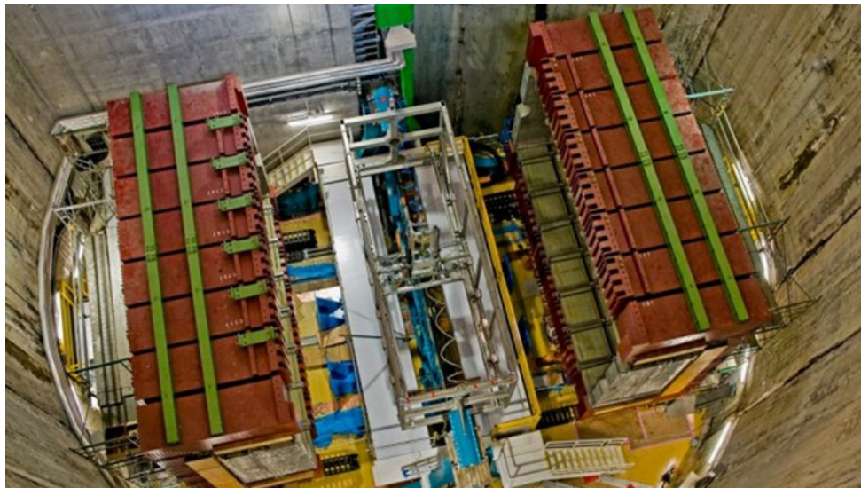
The “pit” 280m after the target station, housing ND280, INGRID, and other near detectors
