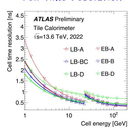
Cell time resolution ~1 ns for cell energy > 4 GeV
