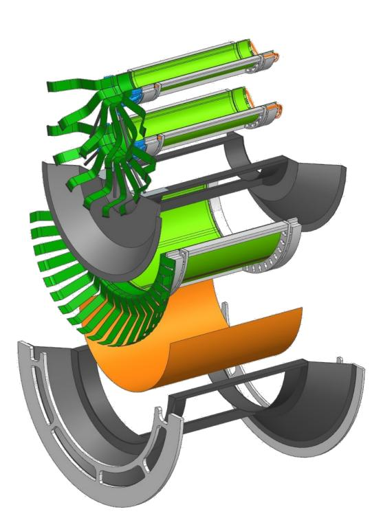
CAD exploded view of IB support with cables and sensors.
