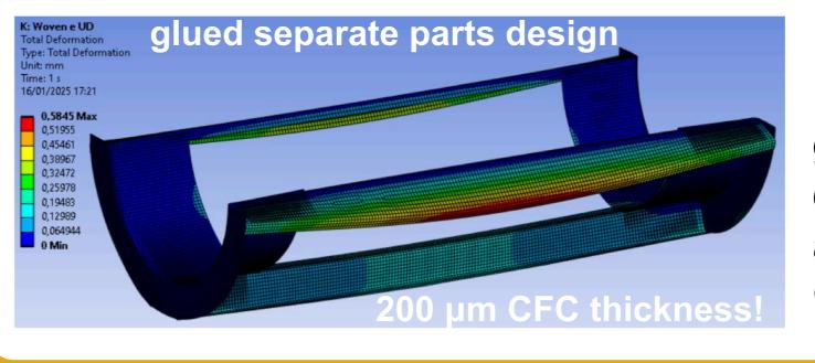
If support is made of separated parts glued together, the deformation is 600  $\mu m$  on edges, due to copper cables, not affecting the sensor region. In this case CFC thickness of 200  $\mu m$  is considered.
