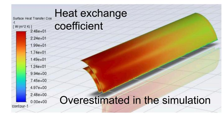
Air flow cooling and possible addition of other cooling elements are still under investigation. Measurements on mock-up with thermal load are needed to confirm the preliminary evaluation of cooling effectiveness.
