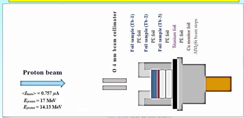
Layout of the experiment to search for multineutron nuclei in a proton induced nuclear reactions on <sup>159</sup>Tb using the stack foil technique
