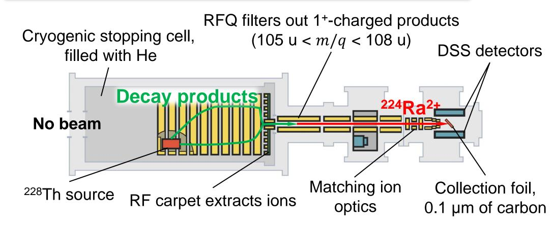
The FRS Ion Catcher (GSI) is a universal system to perform decay and laser spectroscopy and mass measurements of heavy ions. Two double-sided silicon strip detectors (DSSDs) were used to measure charged products of <sup>224</sup>Ra during the **4-month-long** measurement in 2022.
