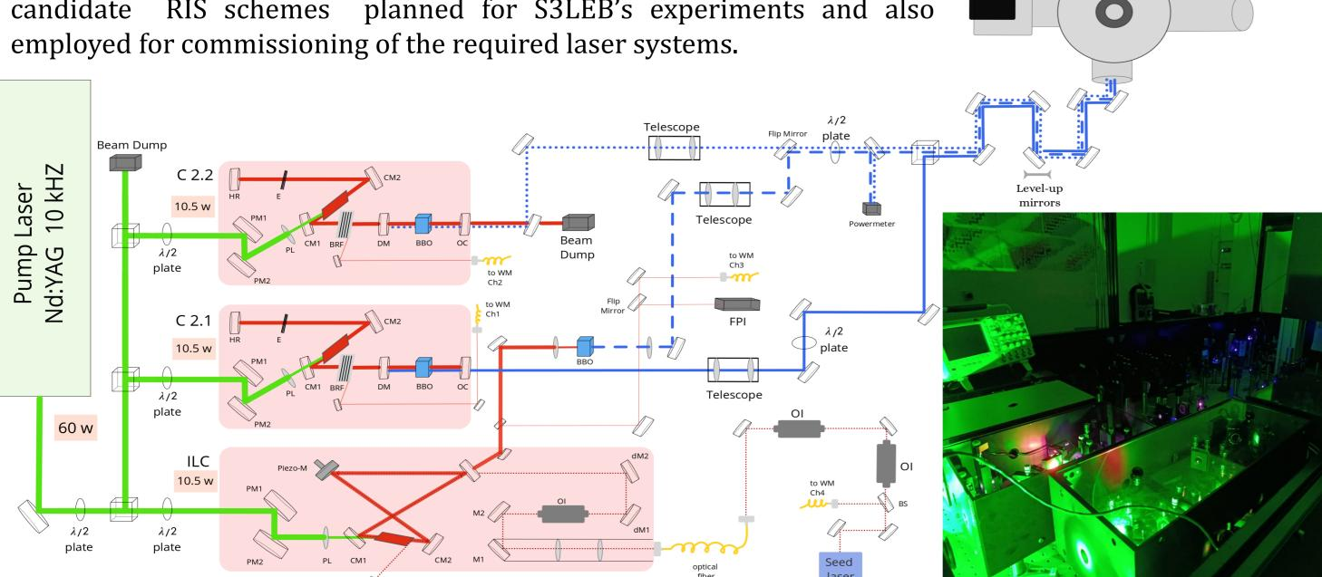
Composed by two mirrors, one of them movable, a Fabry-Perot Laser cavity characterization interferometer (FPI) is a device that transmits light only when the resonance condition is fulfiled allowing to detect the mode structure and the linewidth of the laser systems.
